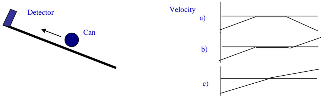
**Figure 1.** A schematic of the rolling can experiment and typical predictions of the time history of the velocity of the can after being launched upward as shown at the left. The audience is usually told that the can starts with negative velocity since it is moving toward the detector. Most believe that the can stops for a finite time before rolling down, and so select a) or b).
